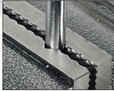
Jaw faces have "V" notches for vertical gripping
