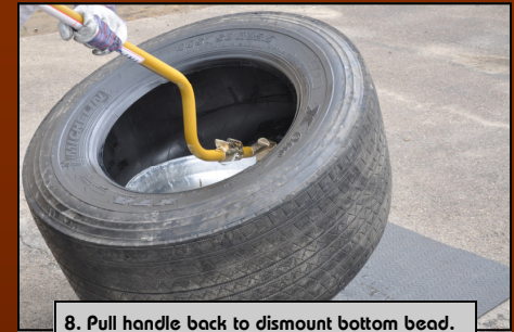
8. Pull handle back to dismount bottom bead.
