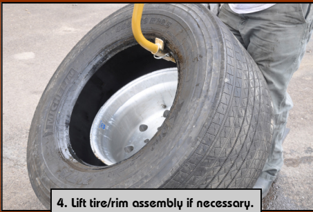
4. Lift tire/rim assembly if necessary.
