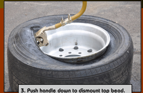
3. Push handle down to dismount top bead.
