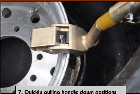
7. Quickly pulling handle down positions tool under bottom bead. See next image.
