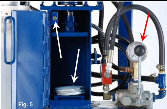
The 3 arrows above point to the Door Safety Switch, Valve Lever Handle and a Crushed Oil Filter.
